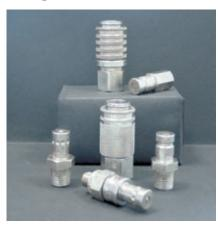
Diagnostic couplings provide easily accessible test points for performance testing of hydraulic systems in plant or on mobile vehicles. This early detection contributes to equipment efficiency and long life. Parker PD & PDP series combine many advantages: ISO 15171-1 & SAE J1502 conformity for wide interchangeability, flat-faced poppet for reduced spillage, possibility to connect under pressure...
