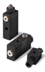
Parker's stackable selector valve is operated by a wet pin solenoid. The valve is capable of switching from one circuit to another at a variety of flows and pressures. If more than two circuits are to be controlled then additional units can be stacked together. Alternatively, the valve can be connected to a pump and used to direct the flow to either one of two different circuits.
