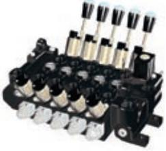
Valves for constant pressure systems are mainly used where operational characteristics are critical and energy consumption is not. In these systems, simultaneous function operation is possible. Valves for constant pressure can return a un-load signal to the variable pump when they are not in use.
