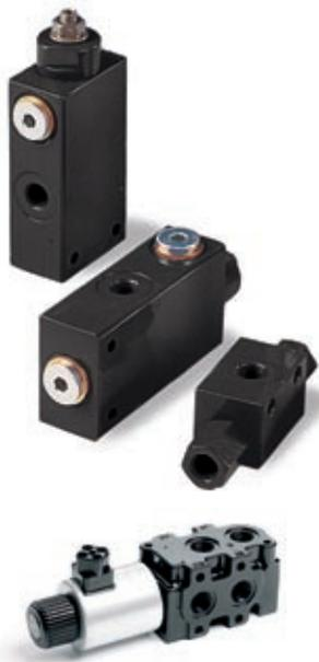
Parker's stackable selector valve is operated by a wet pin solenoid. The valve is capable of switching from one circuit to another at a variety of flows and pressures. If more than two circuits are to be controlled then additional units can be stacked together. Alternatively, the valve can be connected to a pump and used to direct the flow to either one of two different circuits.
