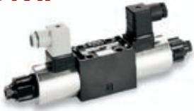
The D1VW is a 3 chamber-, electrically controlled 4/3 or 4/2 way directional control valve. It is activated directly by solenoids with screwed in wet pin armature.
