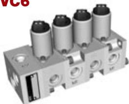
Series PVC6 is a bankable valve assembly used for remote control of directional control valves. The proportional pressure reducing valve creates a pressure proportional to the inlet current. Solenoid Coil Voltage is available in 12 or 24 Volt. The inlet section can be equipped with a pressure reducing valve to protect the control sections (max inlet pressure to control section is 50 bar).
