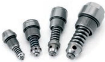
Directly controlled pressure-relief valves with anti-cavitation function. The valves have good pressure characteristics together with very short reaction times. They are compact, tight, reliable and not sensitive to contamination.
