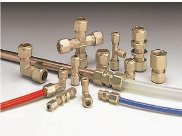
Metrulok is a one-piece ready to use bite type fitting for use with either copper or plastic tubing. The cutting ring is retained within the nut. Metrulok fittings are reusable.
