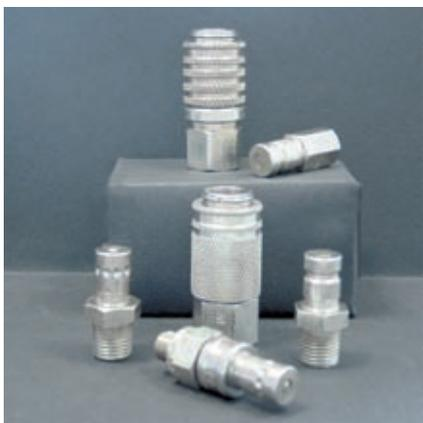
Diagnostic couplings provide easily accessible test points for performance testing of hydraulic systems in plant or on mobile vehicles. This early detection contributes to equipment efficiency and long life. Parker PD & PDP series combine many advantages: ISO 15171-1 & SAE J1502 conformity for wide interchangeability, flat-faced poppet for reduced spillage, possibility to connect under pressure...
