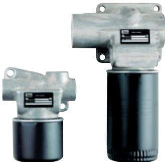
The boost unit provides filtration and make-up fluid to replace pump and motor volumetric losses, while maintaining sufficient pump inlet pressure to avoid cavitation. The semi-closed system could be built with a smaller and lighter reservoir at the same time as, the pump speed is possible to increase. The Boost Units BLA are available in two different sizes:
