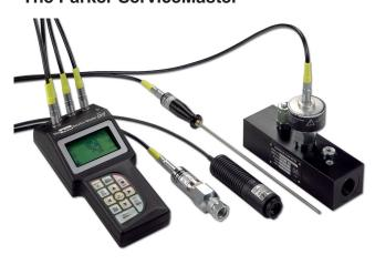
The ServiceMaster is a multi-channel hand meter for the simultaneous measuring of important hydraulic values. All hydraulic parameters such as pressure, differential pressure, flow and hydraulic power can be measured, displayed, stored and processed.
