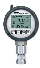
Utilising the ServiceJunior wireless from Parker's SensoControl family of products allows you to comfortably record the pressure values taken from one or several measurement points on your machine or installation. Stored measurement data is transmitted to a PC across distances of up to 150 meters.
