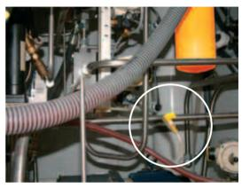
Sampling points should enable extraction of a sample without changing the system's condition. Fine control needle valves are not desirable, as they have a tendency to silt up under some operating conditions, causing the distribution of contaminants in the fluid to be changed. The sampling port should be protected to maintain cleanliness and thoroughly flushed before collecting the sample for analysis. Allow sufficient airspace in the bottle to enable 80% fill.
