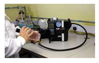
Flush the equipment with the new test sample for 60 seconds prior to starting the test
