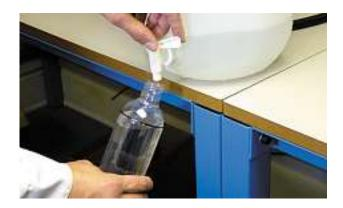
Prior to starting a test, tumble the test portion end over end for 60 seconds to ensure any settled particles are redistributed
