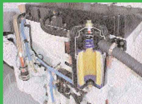
Cummins QSM11 marine engine with CCV cutaway
