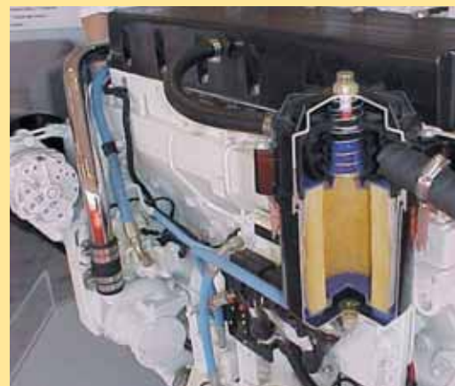
Cummins QSM11 marine engine with CCV cutaway
