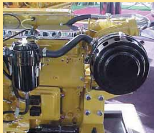
Caterpillar 3196 marine engine with Racor CCV/AF System
