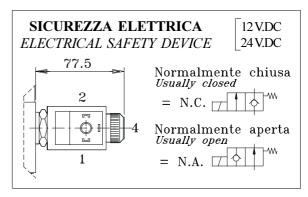
ON - OFF directional control valves with electrical control
