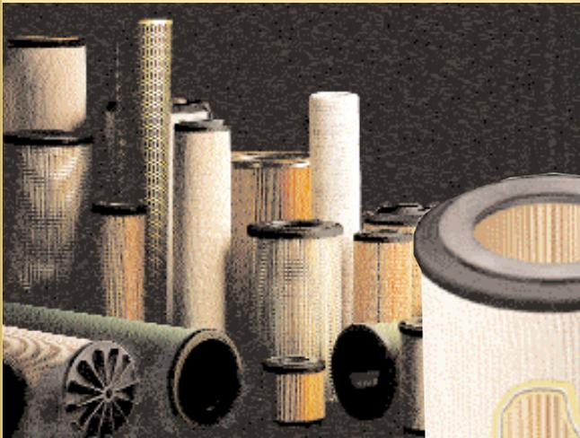
Symmetric layering of high efficiency glass media into depth media can eliminate the need for metal center tubes – even in qualifying coalescer cartridges 75 psi pressure requirements.
