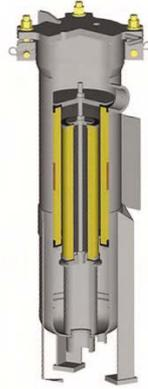
Coalescer and separator mounted in the RVFS housing. Fluid/fuel is passed from the outside of the coalescer to the inside. The coalescer element provides primary filtration of the fuel as well as coalescing free water from it. The clean fuel passes through the separator barrier and into the outlet of the housing. The coalesced water droplets are repelled by the hydrophobic barrier and are collected in the sump of the housing. The sump should be drained routinely.
