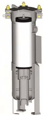
This pictorial shows the mounting of Parker's adaptor and clay canister, FCC-18701. Clay is known as Attapulugus clay, Fullers Earth or diatomaceous earth. The principle use in fuels filtration is to jet fuel. This product can also be used to neutralize acid or products of oxidation from industrial oils; including: hydraulic fluids, lubricating oils, and dielectric fluids.
