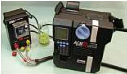
In addition to the Z2 Parker also have the ACM20 laboratory Particle Counter which has been designed in accordance with the Energy Institute (EI) Method IP PM DK.
